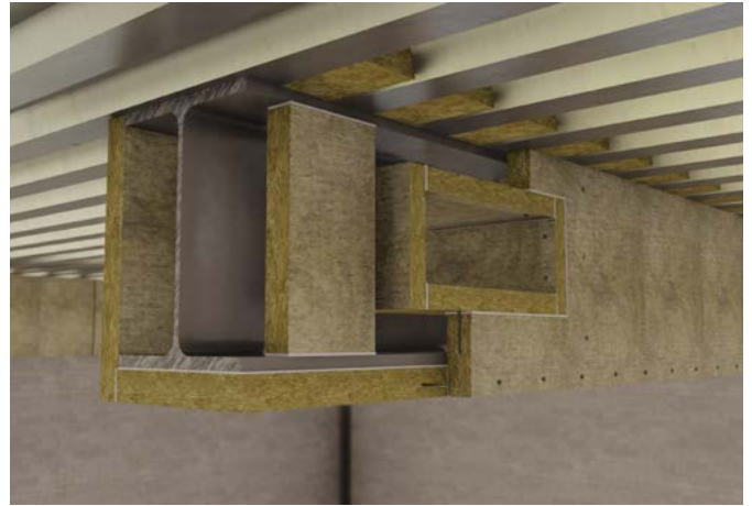
Figure 7 Beam with square or rectangular holes (boxed protection - glued and pinned joints)
